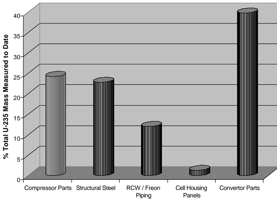
Fig. 7. Percentage of Total U-235 Measured for each Waste Material Type
