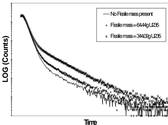
**Figure 8** Decay of fast neutron flux in Hulls Monitor DDA measurement cavity.
