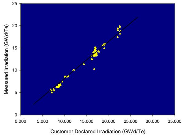
**Figure 6** Measured and customer declared values of irradiation for 80 assemblies from the first THORP campaign of BWR fuel.
