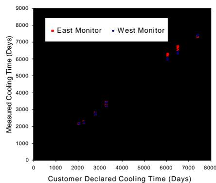
**Figure 3** Measured and customer declared values of cooling time for BWR fuel calibration data.
