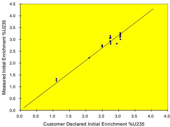
**Figure 5** Measured and customer declared values of initial enrichment for BWR fuel calibration data
