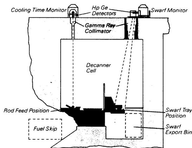
**Figure 1** Mechanical Arrangement of the FHP Cooling Time Monitor and Swarf Inventory Monitor.
