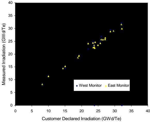
**Figure 4** Measured and customer declared values of irradiation for BWR fuel calibration data.
