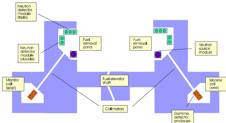
**Figure 2** Schematic Plan View of the THORP Feed Pond Fuel Monitors
