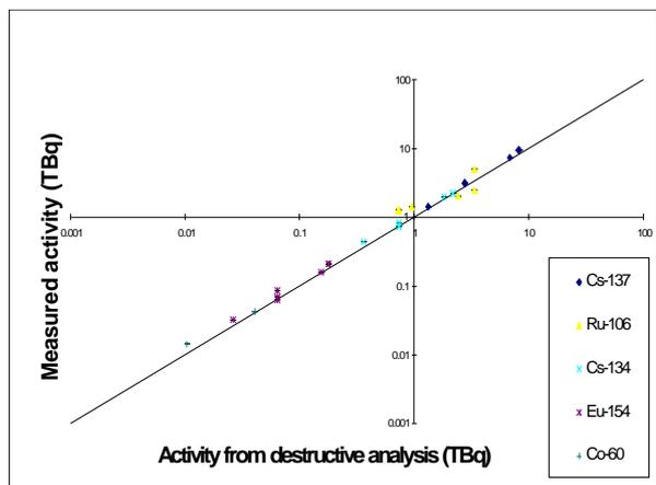
**Figure 10.** Gamma system results measuring spent fuel standards.
