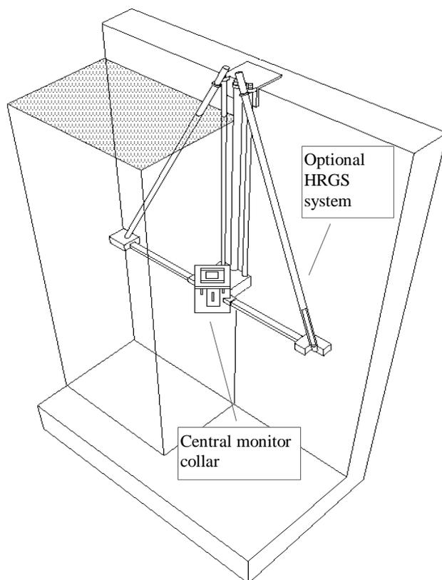
**Figure 11** Burn-up credit monitor configuration.
