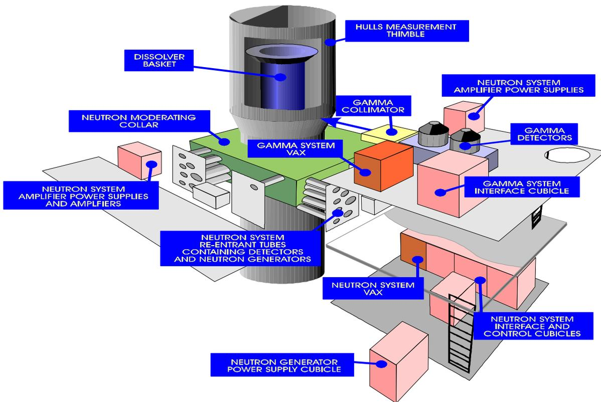
**Figure 7** Schematic Arrangement of the Hulls Monitor.
