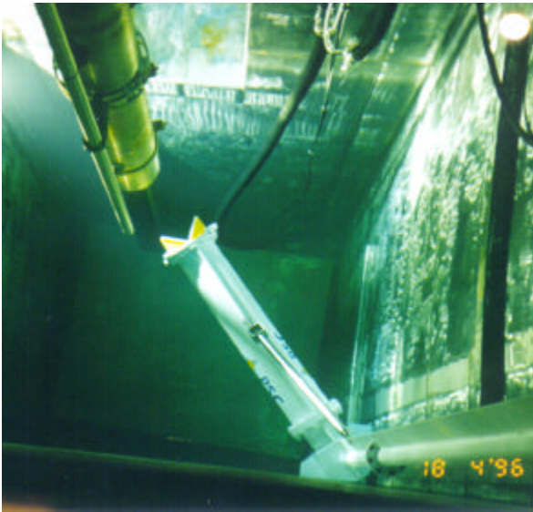
Figure 6. Plan view of gamma collimator and handling machine
