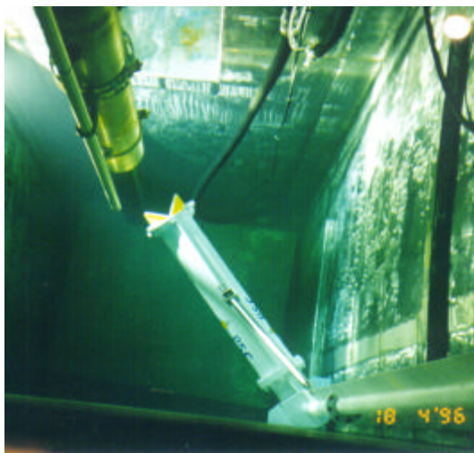
Figure 5 Plan View of gamma collimator and fuel handling machine.
