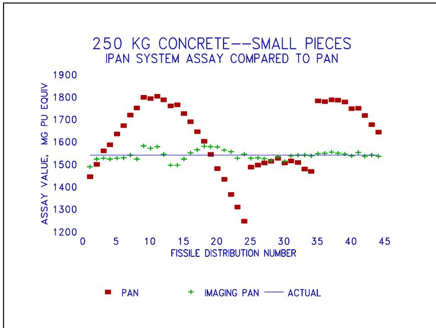
Figure 1: Concrete Matrix Fissile Distributions
